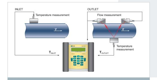
FLUXUS® F601 measures the energy consumed by a system by determining the heat or cold flows entering and exiting the latter (difference method). For this, it is necessary to measure the supply and return temperatures, as well as the volume flow through the consumer system. FLUXUS uses the measured values to calculate the energy flow based on the heat transfer media's enthalpy curves stored in the internal memory.
